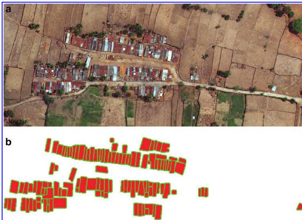
FIG. 4. (a) Sample satellite image of a rural village in India. (b) Ground truth label of the village where red indicates “building,” white indicates “not building,” and green indicates “not sure,” which includes pixels very close to the building boundaries.
