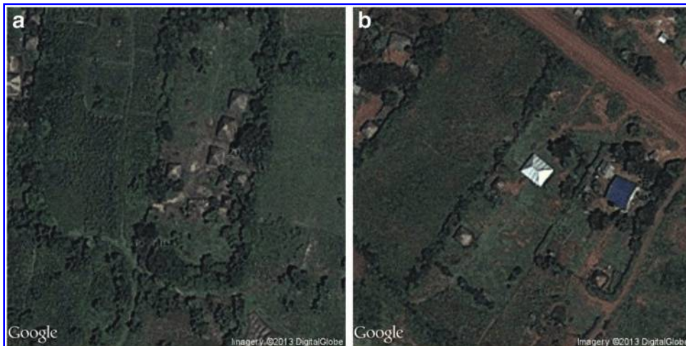
FIG. 1. Sample satellite image patches of the region with (a) thatched roofs in the center and (b) a metal roof in the center.
