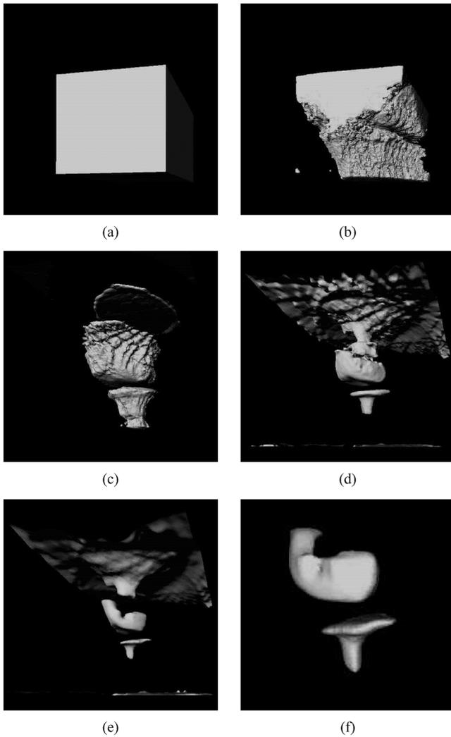
Fig. 3. For  $N = 16$ , (a)–(e) iterations of surface evolution in raster scan order and (f) reconstructed shape of the prosthesis.
