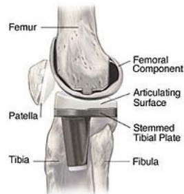
Figure 2: Diagram of knee prosthetic device. Image from Joint Replacement Center at Florida Hospital Celebration Health website ( http://www.celebrationjointreplacement.com ).
