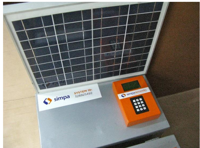
Figure 1. Simpa Networks' solar photovoltaic system.
